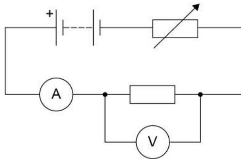
The student recorded how the current in the resistor varied with the potential difference across the resistor.
